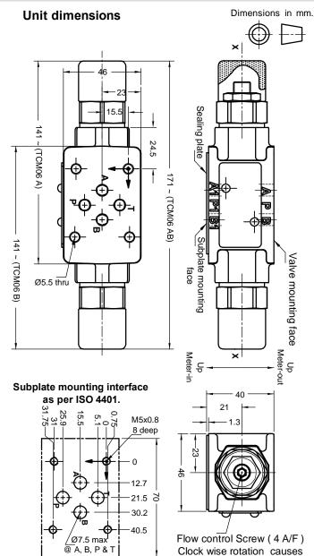
Note: Rotate the valve around horizontal axis 'X' - 'X' by 180° to convert from METER-IN control to METER-OUT control. Valve fixing S.H.C Screws are not in scope of supply. Tightening torque for S.H.C Screws is 16 Nm.
