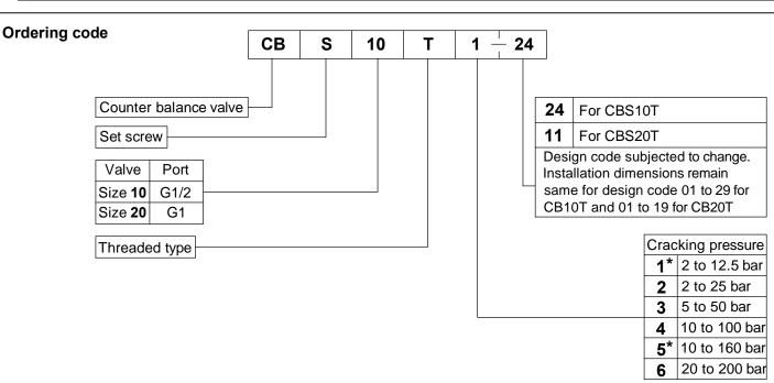
**Note**: Cracking pressure marked with ★ are not available in valve size 20.
